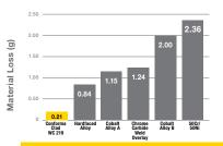
Laboratory testing, following ASTM G73 standards, on low swirl coal spreaders determined Kennametal's WC 219 provides the best erosion protection from fine grit black beauty coal slag. Babcock Power, CCV-DAZ Development Project
